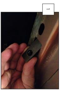
Insert a nut plate for each bracket into the existing holes on the bottom of the body.
