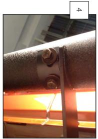
Find the left and right steps; install 2 bolts, with lock washers and washer, through the brackets into the threaded bottoms of the side steps. Tighten down hardware on the body then secure the steps in place.
