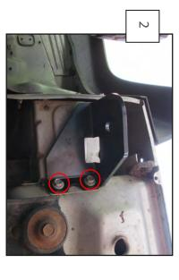
Install (2) of the included 14 mm screws, with washers; in place of the stock screws
