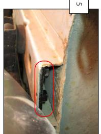
Insert the nut plate into the rail and insert the included (3) 16mm bolts, with washers, through the bracket, through the body and into the nut plate.
