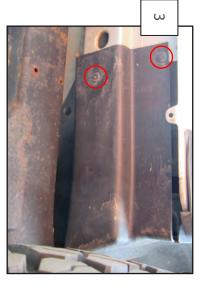
At the rear of the vehicle: remove the (2) plastic push pins, then push the plastic back and out of the way.
