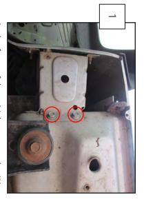
At the front of the vehicle remove the (2) 13mm screws.
