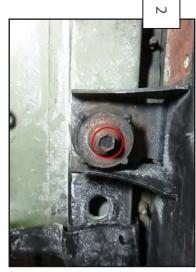
Remove the (2) 16mm factory body bolts, located between the wheels, on one side of the Jeep. (Only remove one side at a time.)
