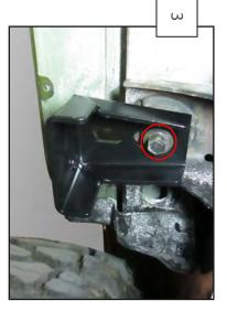
Place a bracket over the front body mount. Reinstall the factory body bolt through the inner oval hole in the bracket. Tighten the bolt until it loosely holds the bracket in place.
