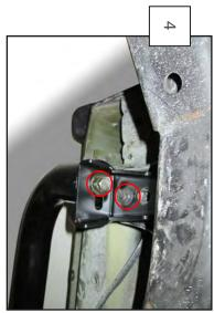
Place a bracket over the rear body mount. Reinstall the stock body bolt through the outer oval hole in the bracket. Tighten the bolt until it loosely holds the bracket in place.
