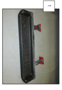
If your Jeep came with a factory step, start by removing the (7) 10mm bolts where the steps attach to the frame. Remove the factory step and repeat on the other side.
