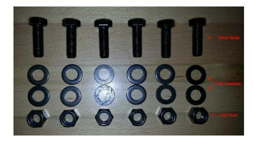
8. Secure the bumper to the bumper brackets on both the driver and passenger side. Each side will require 3 bolts, 3 nuts, and 6 flat washers. Place a washer on the bolt head side and the lock nut side of each bolt. Tighten the bolts with an 18mm socket and use a 19mm or 18mm wrench to hold the nut as the bolt is tightened. Do not completely tighten the bolts/nuts so adjustments can be made during final fitting.
