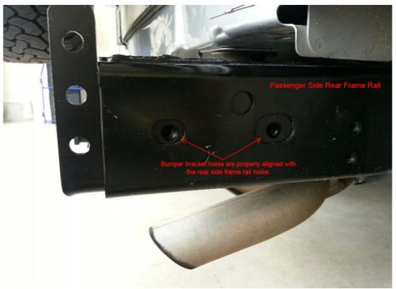
6. Install the 2 hole plates and mounting hardware on both the driver and passenger side frame rails. Place 1 of the 2 hole plates on the outside of the frame rail and align with the frame rail and bracket holes. Secure the plate to the frame rail and bumper bracket with 2 of the supplied bolts. Use lock and flat washers on the bolt head side of each mounting bolt. Do not completely tighten the bolts so adjustments can be made during final fitting.
