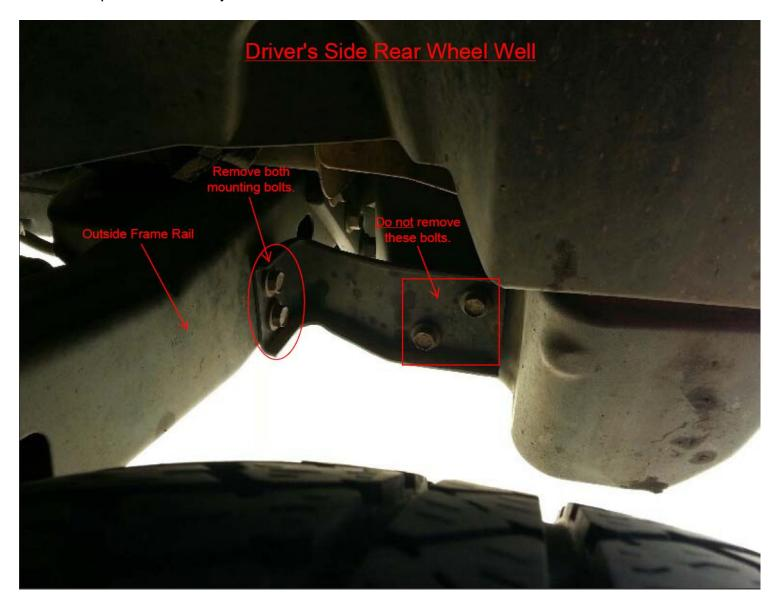
3. Remove the 3- 18mm mounting bolts connecting the tow hook to the driver side rear frame rail. There are 2 located on the side of the frame rail and 1 on the bottom. Place the tow hook out of the way. It won't be reinstalled. The driver side bumper bracket supplied with the kit does not have predrilled holes or welded nuts to allow for the tow hook to be reinstalled.
