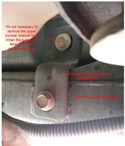
2. Remove the mounting bolts connecting the bumper to the outside frame rail on both the driver and passenger sides. There are 2- 15mm bolts on each side. The bolts are accessible from the rear wheel wells. After removing the mounting bolts the bumper is disconnected from the Jeep. Place the bumper out of the way. It won't be reinstalled.
