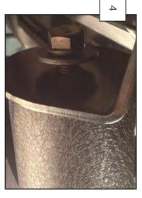
the two 19mm rear bolts Move the bull bar into position and insert
