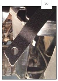
a nut and lock washer. vertical crash bar support and secure it with Bolt Plate that you inserted through the Mount the support bracket onto the Large
