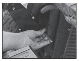
11. Remove the LED light bar and replace the grill by sliding the grill over the brackets and onto the JK. Push in the lower snap pins and replace the upper plastic bolt inserts removed in step 1.
