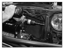
5.1 Use the 1/4-20 one inch bolt and the 5/16 nut as a poor man's nutsert tool to mount the 1/4-20 nutsert
