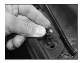
2. Remove the turn indicator lights from both sides (left/right).
