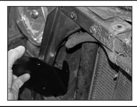
9. Insert the 1/4-20 Phillips head bolts through the mounts and into the nutserts installed earlier (do not tighten all the way down yet).
