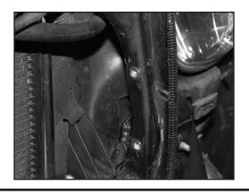
7. See the circle, using a 1/2 wrench, remove the mounting bolt from behind the grill mounting area.
