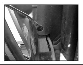
5. Using a drill and a 25/64 (can use a 3\8 size bit) bit to enlarge the holes to fit the threaded nutsert.
