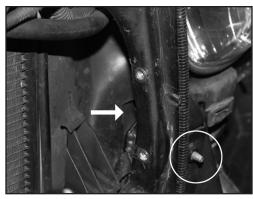
8. Slide mounting brackets into place, insert and hand tighten the bolt (do not tighten all the way down yet).
