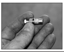
6. Insert the nutsert into the hole that was enlarged in step 5. Tighten down until it is snug or tight within the hole. (hold the 5/16 nut with an open end wrench while using a xxxxxxx socket to tighten the nutsert into the hole.
