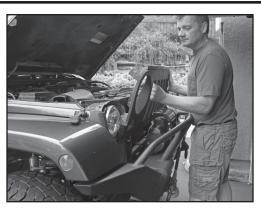
12. Replace the turn indicator lights into both sides (left/right).
