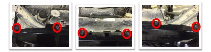
6. Insert the self-tapping screw into the Wild Boar Grille and into the chassis.
