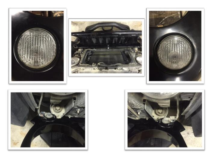
5. Place the Wild Boar Grille back onto the Jeep and insert the six plastic clips into the grille and upper cross member.
