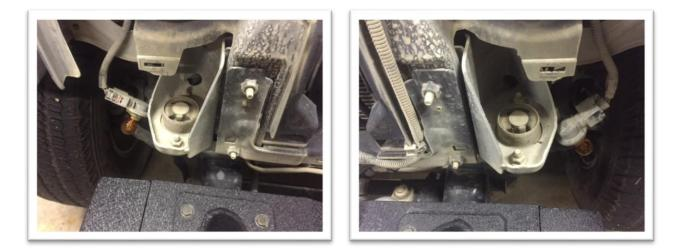
Place the Wild Boar Grille onto the Jeep to mark the place on the chassis and the grille that will be drilled. Remove the Wild Boar Grille and drill a hole in the chassis where the mark was made. Then drill the hole into the grille.
