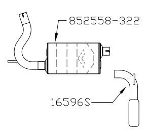
Installation diagram for: SYSTEM #817693 2012-2014 JEEP WRANGLER JK 2 & 4 DOOR • 3.6L V-6
