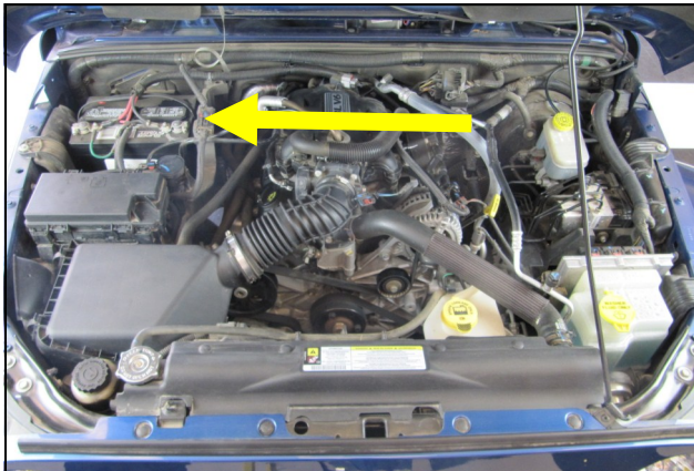
1. Disconnect The Negative Battery Terminal! It's recommended to allow the engine to fully cool down before starting the intake installation.
