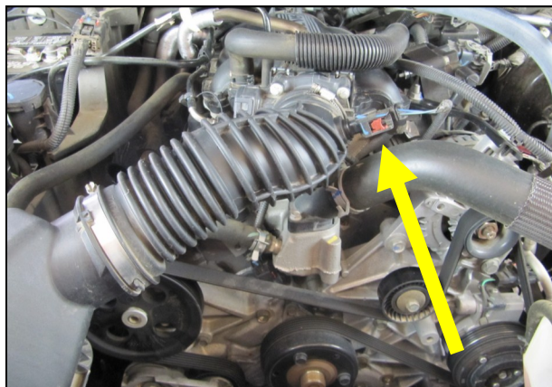
2. Disconnect the air temp sensor in the factory intake. loosen the clamps on both ends of the tube and remove it from the vehicle.
