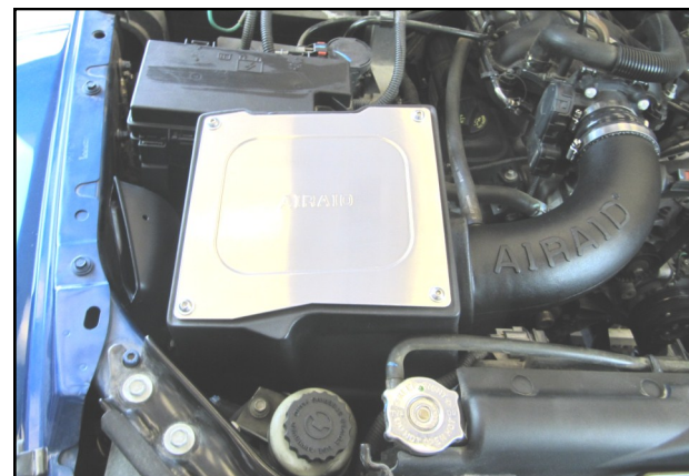
18. Double check your work! Make sure there is no foreign material in the intake path. Make sure all clamps, hoses, bolts, and screws are tight. Double check the hood clearance!
