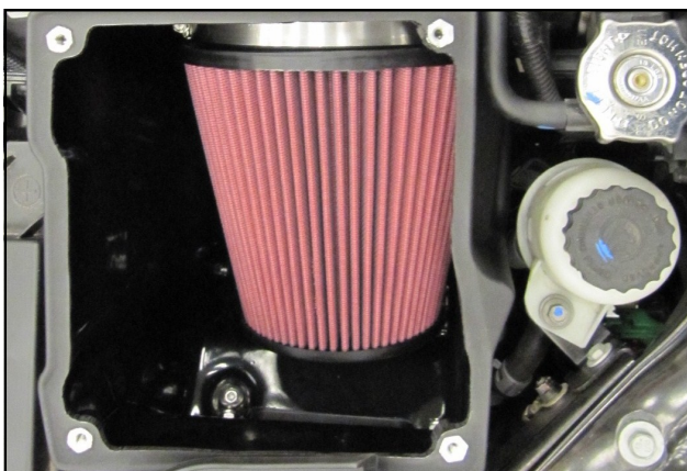
16. Slide the Airaid Premium Filter onto the Intake tube inside the Cold Air box and tighten the clamp.
