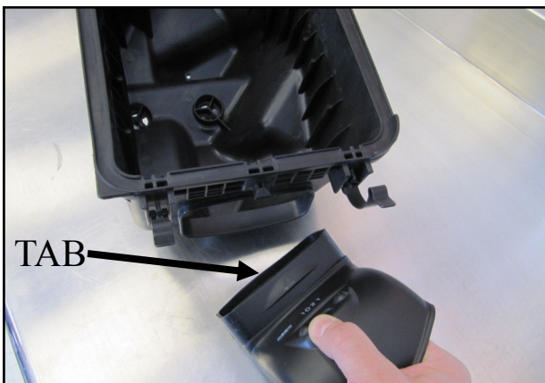
5. Depress the locking tabs holding the factory air scoop in the lower half of the airbox and remove it.
