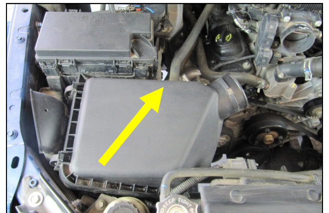
3. Disconnect the crankcase breather line from the top of the airbox. Remove the entire airbox as an assembly by unseating it from the mounting grommets in the inner fender and lifting upward.
