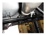
4) Place a provided clamp onto the slip-fit of exit pipe **#86127S** and slide onto the back of over-axle pipe **#86126S**. Connect the hanger on the pipe to the rubber mount on the vehicle and tighten the clamp enough to hold, but still allow for adjustment.
