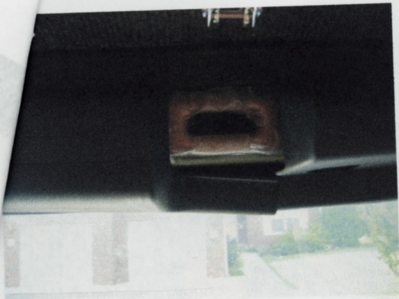
7 Disengage soft top from windshield.
