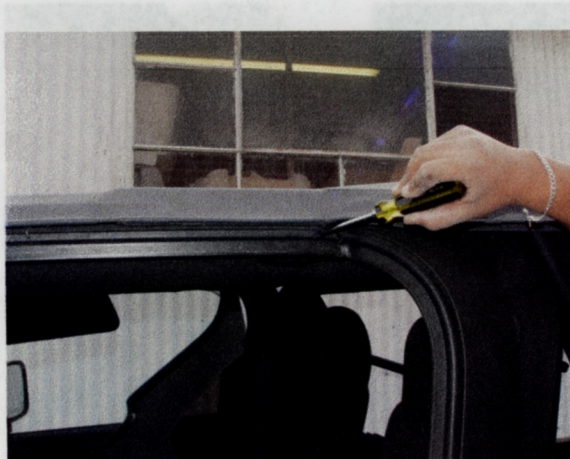
5. Pry open side connections with screwdriver
