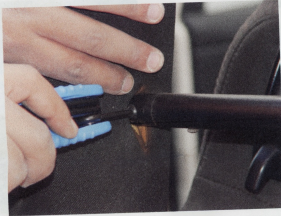
9. Remove bolt from soft top frame.
