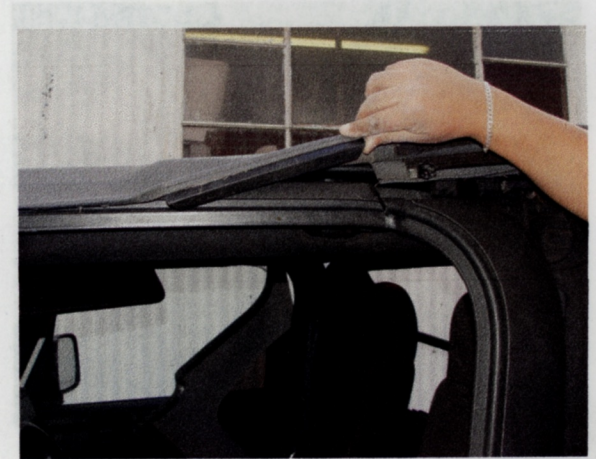
6. Remove side connections to door frame.
