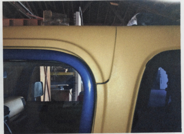
23. It should look like this after the flange bolts are tighten. you can make adjustments by moving the back section front to back.
