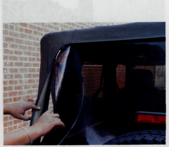
2. Unzip rear window and remove.
