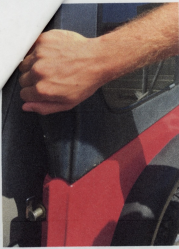
24. Pull out the front flush to the body, tighten bolt. Now tighten the remaining bolts
