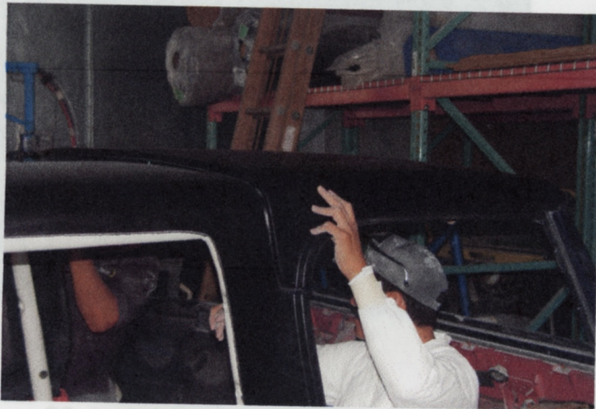
16. Using 2 or more people put the rear section on, followed by the front section. Do not put bolts in yet.
