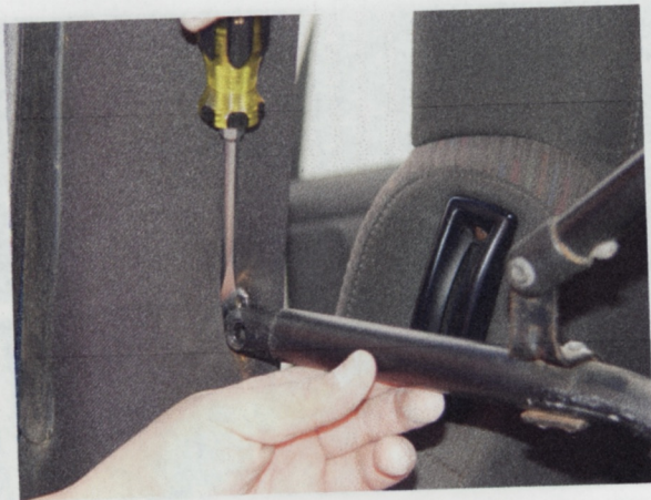
10. Pry off soft top frame from roll bar
