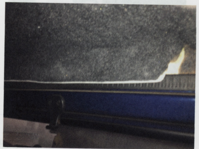
17. Sit in the front seat. Make sure the windshield stop is not hung up on the molding. It should look like this.
