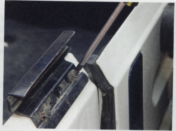
13. Remove rear bar holders.
