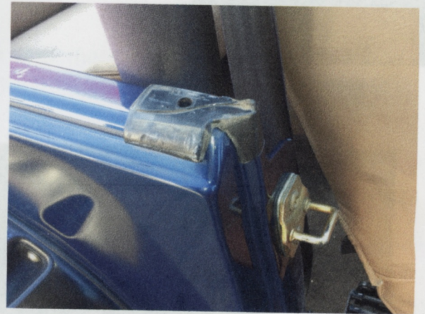
15. Do not remove front corner seal.
