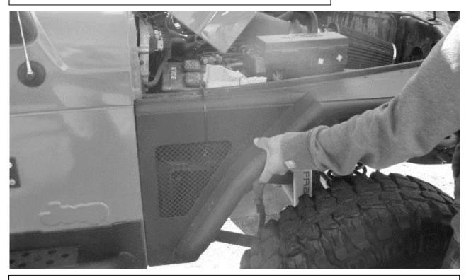
Step 1 Place the new fender on to the jeep. Note: If the new fender does not seem to fit grind excess material from the original fender.
