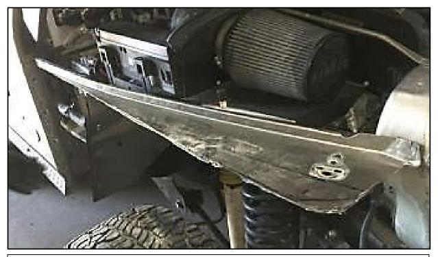
Step 7 When the cut metal parts are all removed, your modified fender should look like the picture above.
