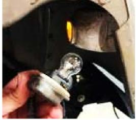
Step 2 Twist and unplug the signal lights from the fender. As shown above.
