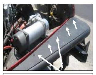
Step 5 Using the holes in the new fender as a guide Drill Five (5) 1/4 inch holes through the factory sheet metal.
