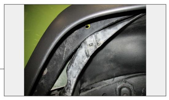
Pull back the fender liner from the lip of the fender. Squeeze the well liner retainer tab and push it back through the fender. Remove any other hardware holding the wheel well liner in place.
