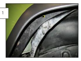
Pull back the fender liner from the lip of the fender. Squeeze the well liner retainer tab and push it back through the fender. Remove any other hardware holding the wheel well liner in place.
