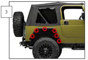
Reinstall (6) of the (8) 8 mm screws that were removed. (5) of the plastic nuts will be reused and 1 screw will thread into the body.
