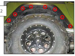
Remove the (8) - 8 mm screws holding the fender flare to the body. Insert the adjustable wrench behind the body to hold the square plastic nut while removing the 8 mm screw with a socket wrench. The front 2 screws thread into the body.
