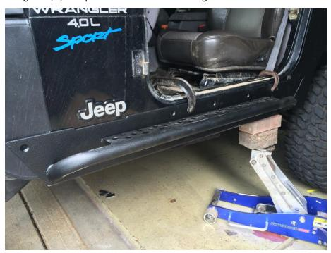
6. Using the holes in the rocker guards as guides, use the 13/32" drill bit and drill holes through the body of the vehicle.
