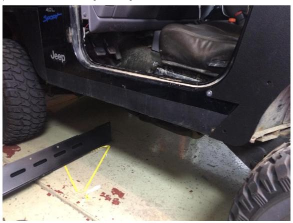
2. Locate two rear body mounts. Loosen two rear body mount bolts using a 16mm wrench. (Body mounts can often be very rusty. Spraying bolts with penetrating oil in advance can break up rust and aid in the prevention of the bolts from breaking during loosening).
