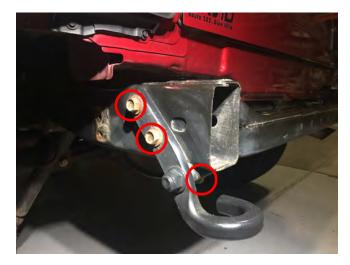
**STEP 2** // Remove the (3) 15mm bolts securing the tow hook to the driver side frame rail.
