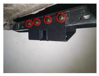
STEP 5 // From under the vehicle, install the (1) Tow Hitch to the frame using the (4) M12 x 120mm bolts, flat washers, lock washers, and nuts. Torque to 40 ft - lbs.
