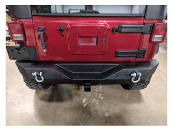
$\ensuremath{\text{STEP 6}}$  // Insert the (2) D-Rings if desired. Installation is now complete.
