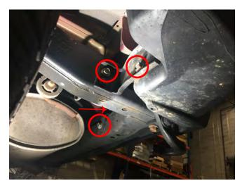
**STEP 1** // Remove the (4) 15mm bolts on the outside of each frame rail. Then remove the (4) 15mm bolts securing the plastic bumper to the frame. Remove the bumper.
