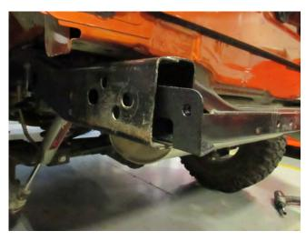
**STEP 3** // Insert the (2) frame rail brackets into the frame rails. \*\*Note be sure that the holes from the frame rail line up with the bracket holes.
