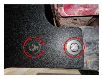
**STEP 4** // Install the new Barricade bumper to frame rails using the (2) M12 x 40mm bolts, flat washers, and lock washers. Torque to 40 ft - lbs.
