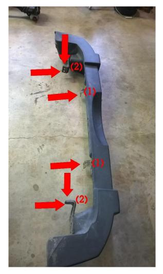
3. To remove the factory hitch receiver (if equipped) remove the (4) 18mm mounting bolts.
