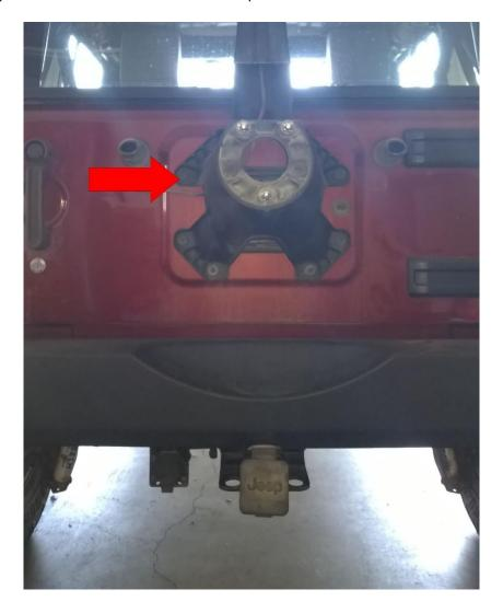
2. Remove the six mounting bolts from the stock bumper using a 16mm socket. Pull up and out to remove the
