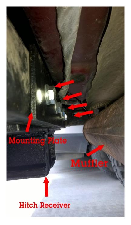
8. Secure the bumper to the frame using the corresponding hardware
