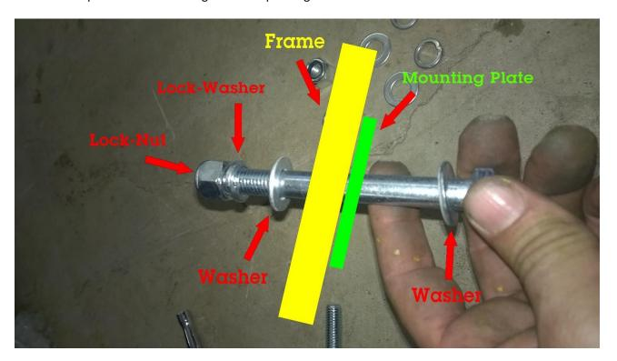
9. Tighten all of the bolts and the installation of your Barricade Trail Force HD Rear Bumper is complete.
