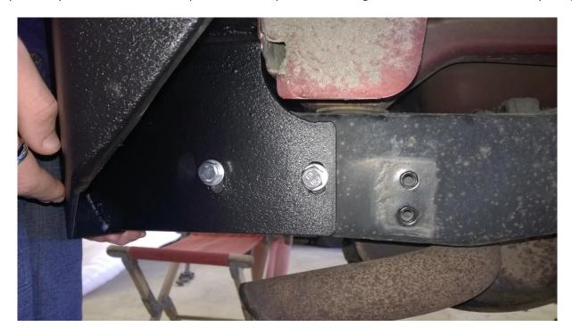
7. Next, install the metal mounting plate on the back side of the frame using the (4) long 18mm bolts and the corresponding washers.
