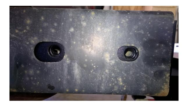
6. Slide the bumper into place, align the holes, and secure it to the frame using the (4) short 18mm bolts and corresponding washers provided. Do not fully tighten until the entire assembly is complete. (Note: the two holes previously used for the stock bumper will be left open for mounting a Barricade roof rack or other option.)
