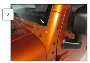
Remove the (6) torx head bolts shown above. Be sure to secure the panel with one hand while removing the last bolt, the panel is heavy and may fall away from the car on its own.
