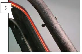
Feed the wiring through the remaining vertical windshield mount into the desired location. Once your wiring is routed properly, first slide the top of the bar into the horizontal section and loosely install the provided nut, bolt, and washers. Next, install the windshield mount. Double check that everything is aligned properly before tightening the rest of the hardware in place.
