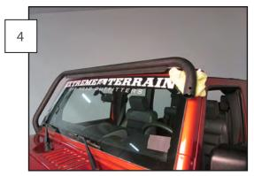
Start by mounting the vertical windshield mount first on the side that will not carry any wiring, followed by the horizontal bar. It's recommended to install and route the wiring through the open end before installing the horizontal bar. Keep all hardware loose at this point.
