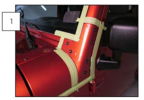
The light bar sections are large and can be awkward to handle. It is recommended that you cover the area surrounding the windshield mount with painters tape to help protect from any scratches during installation.
