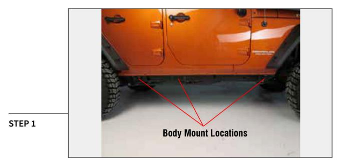
Begin by locating the body mounts that run along the frame of the vehicle. There are (3) for 4-doors, and (2) for 2 doors.
