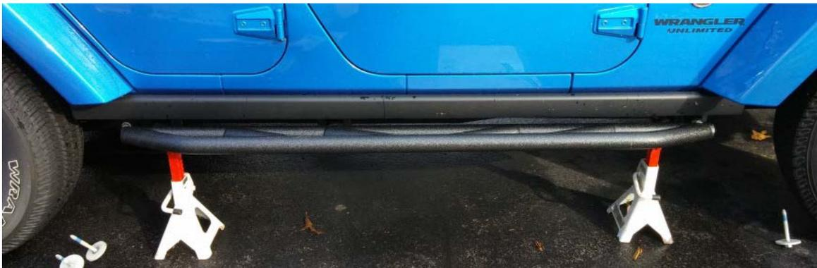
8. Following the instructions, put the blue Loctite on the bolts. Slide the bolts back into place through the mounting holes in the sliders. Finger tighten the bolts into place and then tighten a few turns with the wrench.
