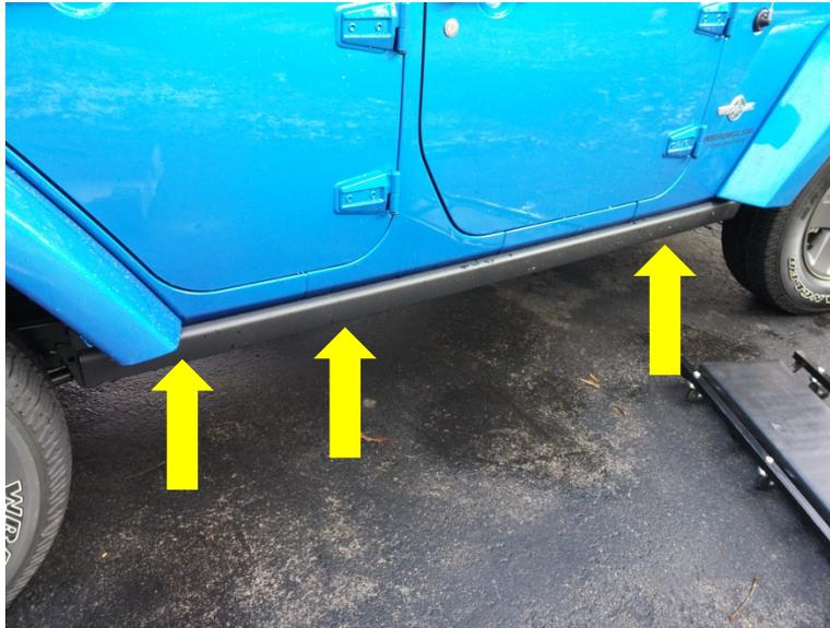
4. Using the 18mm socket, loosen the bolts.
