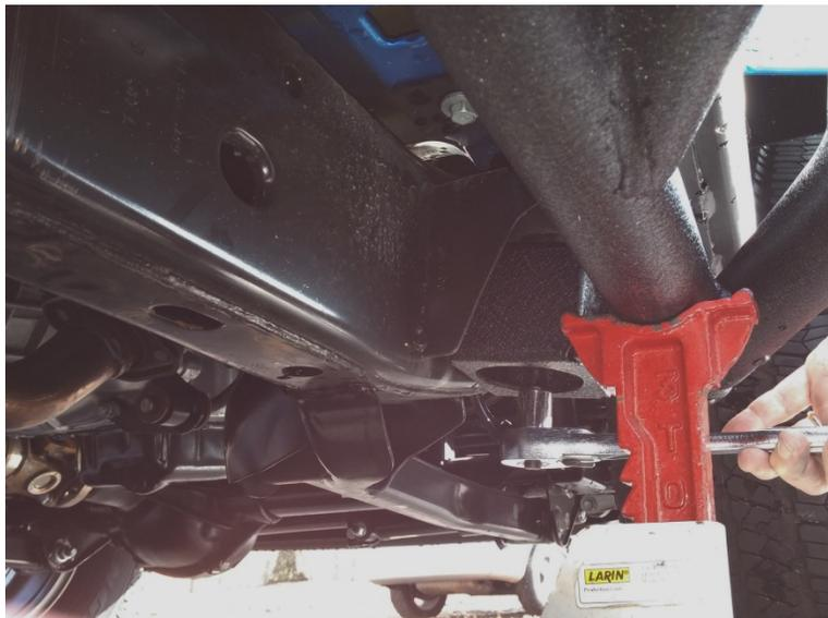
11. Use the torque wrench to tighten the bolts to 35 lb-sq ft.
