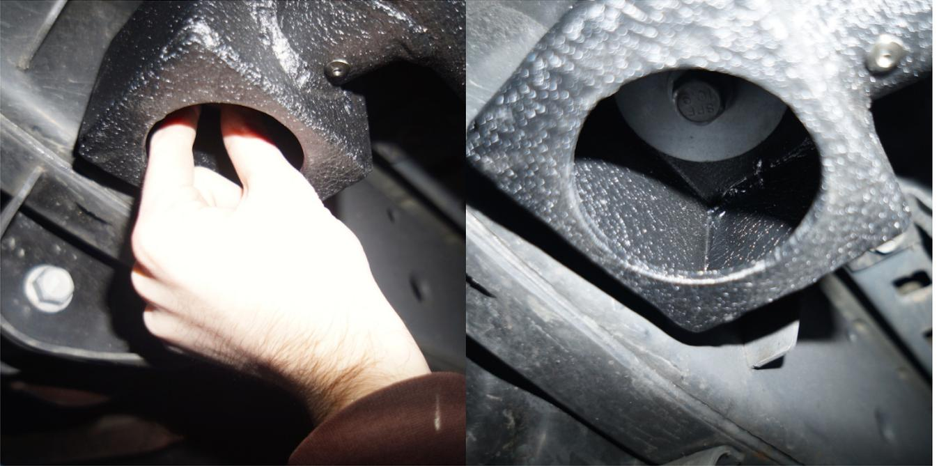
5. Torque each of the bolts to factory spec (35 ft\*lbs) in an in several intermittent steps while alternating between bolts. Do not torque one bolt fully then torque the other fully. **Warning:** These bolts are tapered; if you crank one down all the way first and then attempt the other you may strip out the threads.
