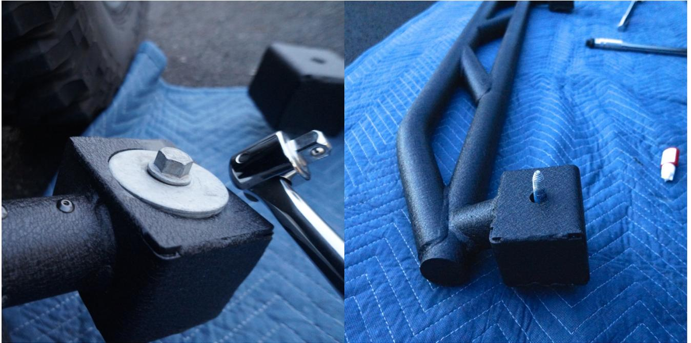
3. Apply some blue (semi-permanent) thread locker to the threads.
