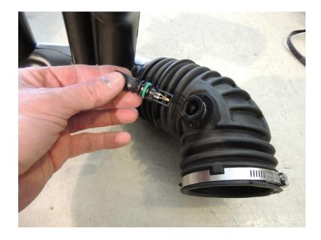
• Transfer IAT sensor over to new intake tube.
