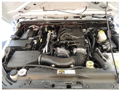
• Unplug your factory IAT sensor located on the bottom of the intake tube.
