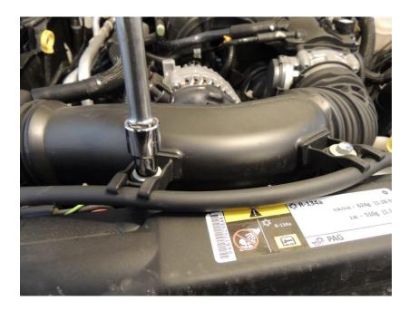
• Loosen hose clamp holding the intake tube to the throttle body.
