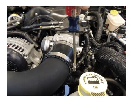
• Bolt intake tube to heat shield using supplied spacer, washers and nuts.
