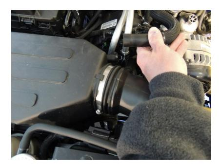
Remove the two bolts holding intake tube to fan shroud
