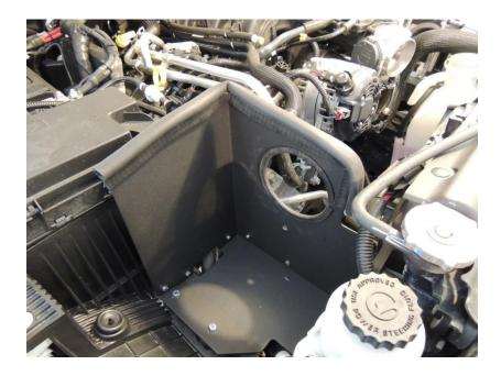
• Remove IAT sensor from factory intake tube.
