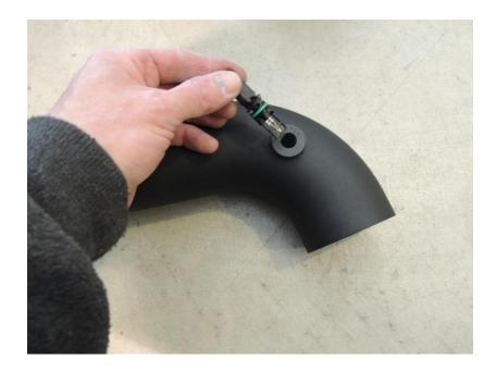
Install intake tube to throttle body using supplied coupler and hose clamps.
