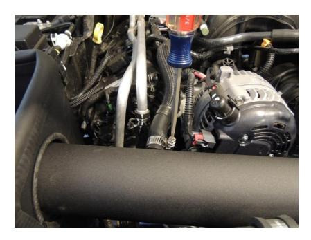
• Install new air filter and secure into position using the supplied clamp.
