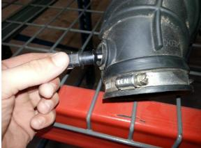
**Step 6:** Install the IAT sensor into the new intake tube assembly.
