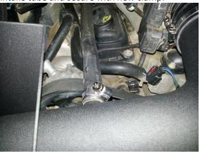
**Step 14:** Plug in the IAT sensor that you previously installed into the intake tube.
