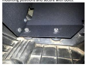
**Step 10:** Add the supplied rubber gaskets to the top of the heat shield and in hole for the intake.
