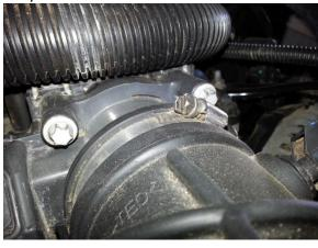
**Step 4:** Pull the entire intake assembly up and away from the vehicle.
