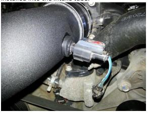
**Step 15:** Install the filter and tighten down using the supplied hose clamp.
