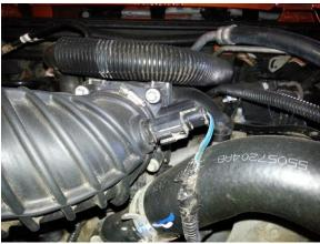
**Step 2:** Slide the PCV hose off of the factory air hose.
