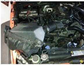
**Step 5:** Remove your factory IAT sensor from the factory intake tube.
