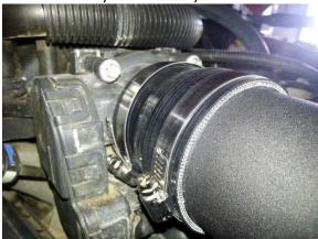
**Step 12:** Secure the intake tube to the heat shield using the supplied spacer.
