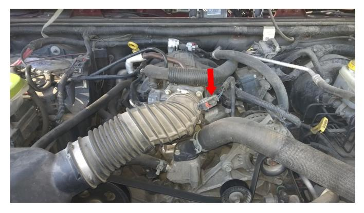
2. To unplug the IAT sensor, slide the red lock-clip up and squeeze the ends of the plug while gently pulling up.
