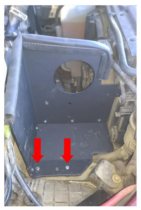
11. Install the large rubber gasket on the top of the heat shield and small gasket in the intake tube hole.
