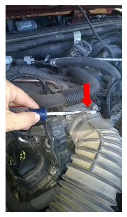
5. Pull the entire factory cold air intake up and away from the vehicle. (It is not bolted on. If you wiggle it a little the three clips shown below should release easily.)
