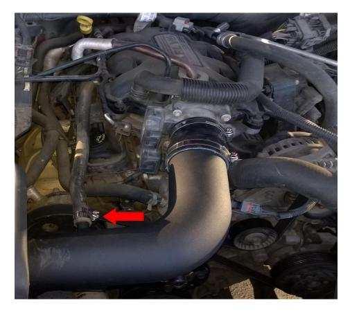
16. Plug in the IAT sensor that you previously installed into the intake tube.
