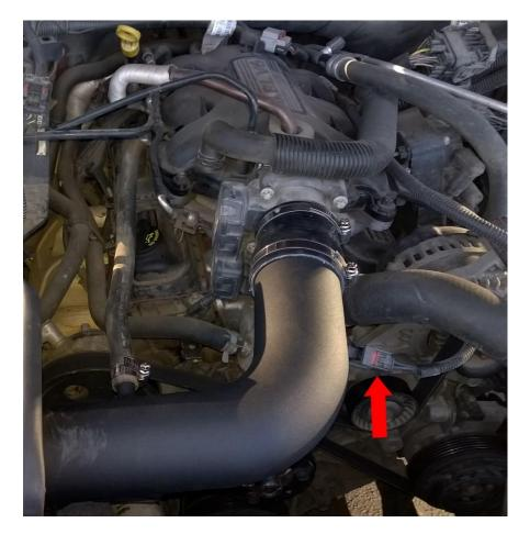
17. Tighten the heat shield mounting bolts, then install the filter onto the new intake pipe and tighten down using the supplied hose clamp.
