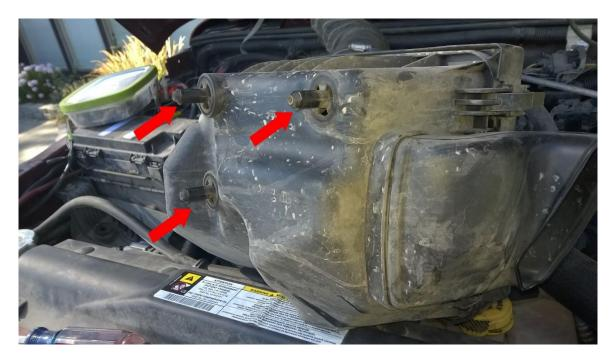
6. Remove the IAT sensor from the factory intake tube. Using a flathead screwdriver gently pry it up being careful not to damage the sensor.
