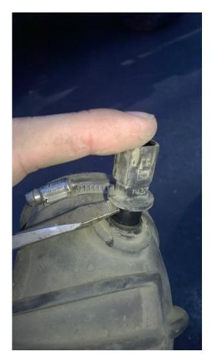
7. Install the old IAT sensor into the new Red Rock 4x4 intake tube. Being careful not to damage the sensor, gently press it into the rubber grommet using a twisting motion.
