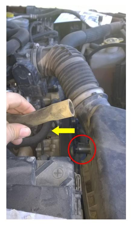
4. Using a flathead screwdriver, remove the hose clamp holding the intake tube to the throttle body.
