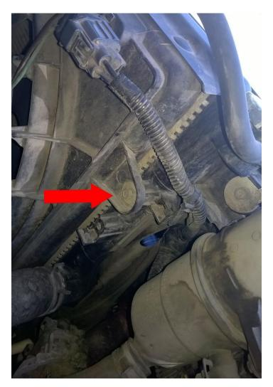
10. Install the heat shield using the factory mounting positions and secure with 10mm bolts. (The nuts can be attached by either removing the factory inner fenders, or by turning your wheels to make the bolts easier to reach.) Note: You will only use two of the original mounting holes.
