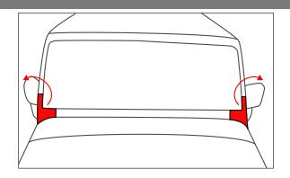
2. Attach left and right brackets to front crossbar with supplied M10x60 bolt and nylon lock nut. Do not tighten completely to allow for adjustment.
