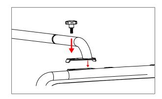
12. Mark and drill 3rd hole for the rear brackets using a 5/16" bit. Use supplied self-tapping screw for the 3rd hole. Adjust the rack to the best position and tighten all bolts.
