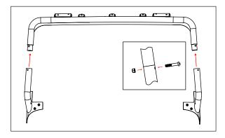
3. Install front crossbar assembly to vehicle using factory hardware retained from Step 1. Do not tighten completely to allow for adjustment.
