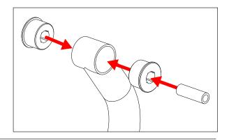
7. Place rear tube into hinge bracket. (There are Left-hand and Right-hand sides; tube should bend in towards fender flare.) Insert the M12x85 bolt through the hinge and bushing sleeve, and into the weldnut. Tighten bolt. Repeat for both sides.
