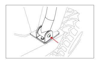
8. Install rear crossbar with supplied M10x65 bolts and nylon lock nuts. The tube horn openings will face the front of the vehicle. Do not tighten completely to allow for adjustment.
