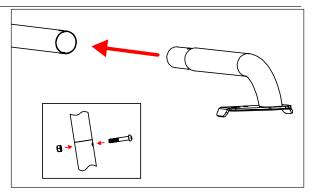
11. Locate the front brackets on the receiving plates of the front crossbar. Use supplied quick release knobs to connect the tiltable section to the lightbar portion.
