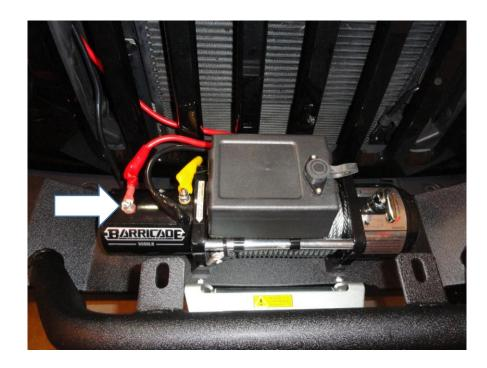
b. Short black wire with yellow jacket from the control box to the yellow terminal (white arrow) on the winch motor.
