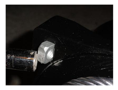
2. Set winch on bumper, lining up holes in winch with holes in bumper. Install four ¾ inch mounting bolts from bottom side of bumper using ratchet and 5/8 inch socket, torque to 35-40 pounds.
