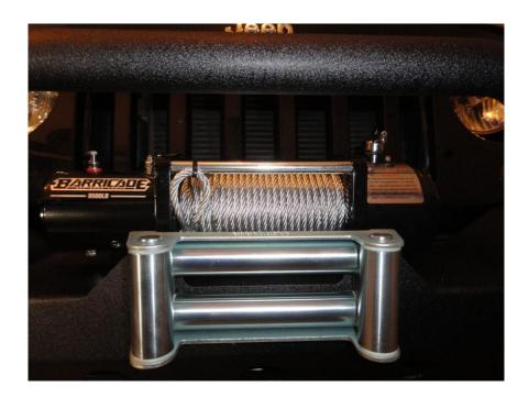
4. Mount control box on top of winch rails using bracket, tightening two set screws with offset screwdriver. Attach control box wires and supplied long black wire.
