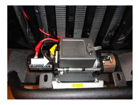
d. Thin black wire from the control box to the bottom terminal of the winch motor.
