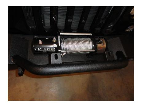
3. Mount fairlead (winch cable guide) in bumper slot using two supplied bolt/nut/washer sets.
