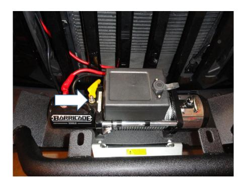
c. Short black wire with black jacket from the control box to the black terminal (white arrow) on the winch motor.
