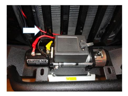
f. One end of the supplied long black wire (white arrow) to the bottom terminal of the winch motor (sharing this terminal with the thin black wire from the control box) and the other end of the supplied long black wire to the negative terminal of the battery.
