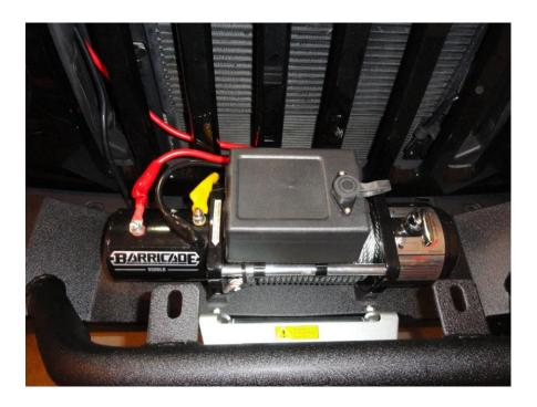
a. Short red wire from the control box to the red terminal (white arrow) on the winch motor.
