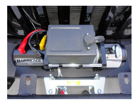
5. Route long red wire from control box and supplied long black wire from winch motor to battery. Attach the red wire to the positive battery post and attach the black wire to the negative post of the battery.
