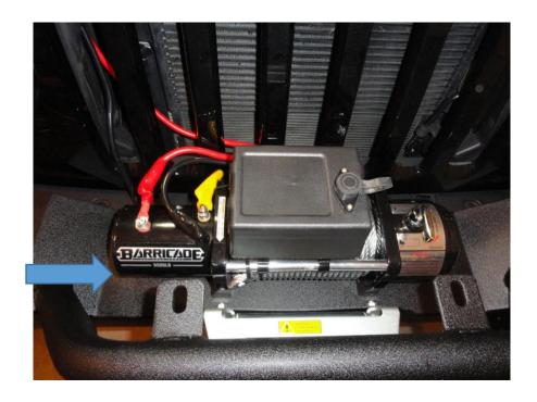
e. Long red wire from the control box to the positive terminal of the battery.
