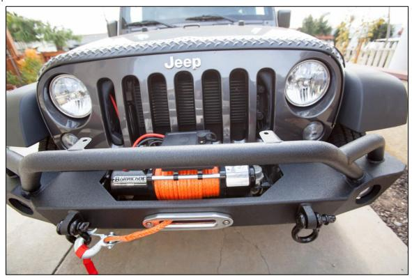
2. Unpack the Barricade Winch Cover and remove any stickers. Gently lift your winch cables up and away from the front grill of the Jeep. Fully open the bottom of the Barricade Winch Cover by releasing and relocating the securing device on the string to the end of the string. Place the Barricade Winch Cover over the Barricade Winch and pull the cover down around all sides of the winch.
