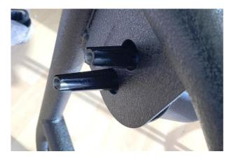
3. If the replacement mirror is mounted to the factory door, secure into position with the factory T40 Torx bolts. If the mirrors are installed on Tube Doors, use the supplied hardware from the kit to secure into position.
