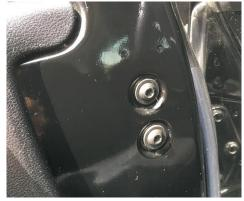
2. Insert the appropriate side, replacement mirror into position. The photo below illustrates the mirror mounted to an aftermarket Tube Door, this highlights the mounting stems that would not be seen in a factory door installation. **Note:** if the Jeep is equipped with wiring for the mirror, attach the factory wiring before inserting into position.
