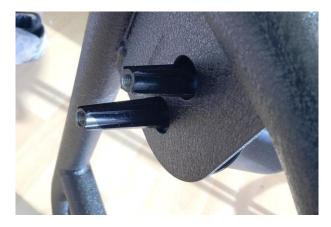
3. If the replacement mirror is mounted to the factory door, secure into position with the factory T40 Torx bolts. If the mirrors are installed on Tube Doors, use the supplied hardware from the kit to secure into position.
