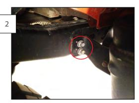
Remove the 4 stock 15mm stock bumper mounting bolts that are located on each side of the frame.
