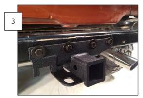
IF YOUR WRANGLER HAS AN EXISTING HITCH: After removing the stock bumper; the hitch bolts are accessible. Remove the 4 hitch bolts that extend through the frame.
