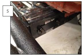
Lay the plate on the outside of the frame and insert 2 bolts through the plate, the frame and into the threads on the bumper.
