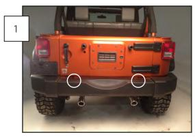
Remove the 2 upper stock 15mm, bumper bracket, bolts from underneath the vehicle.
