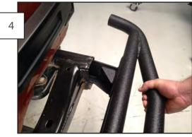
Place the new bumper into the ends of the frame rails and hold it level. Have someone hold the bumper level while you tighten the bolts. If you are installing this bumper yourself, you can hold the bumper with one hand while tightening down the bolts.
