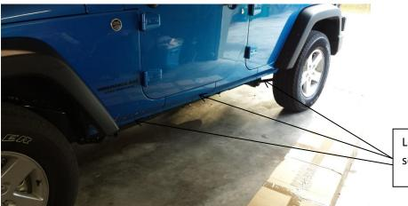
Location of the 6 holes in the pinch seam.
