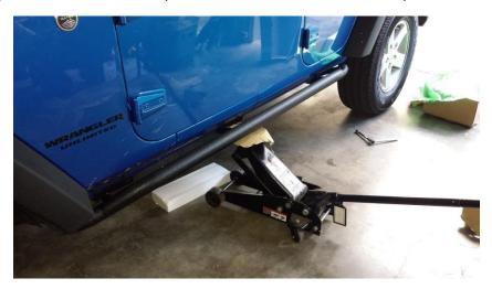
6. Insert a 10mm bolt with a small washer through the front hole and the rear hole with another small washer and the nylon lock nuts on the bolts. (Don't tighten the bolts. Just a few turns to hold them up securely). Now you can let go of the rocker guard (lower the floor jack) as it will be suspended to allow you install the other bolts.
