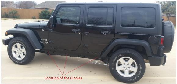
2. First locate the 6 holes on the side of the vehicle in the pinch seam at the bottom.
