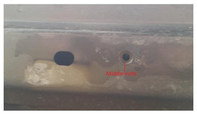
4. While holding the rail in place insert the middle 13mm bolt with the large washer and tighten, but do not tighten the bolt all the way.
