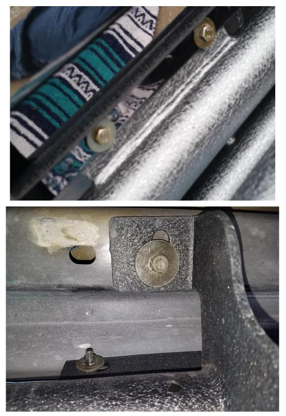
7. Using either two socket wrenches with two 10mm sockets, or a single socket wrench with a 10mm socket and an open ended 10mm wrench; tighten all six nut/bolts on the pinch seam.
