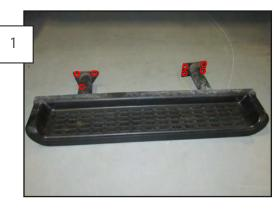
If your Jeep came with a factory step, start by removing the (7) 10mm bolts where the steps attach to the frame. Remove the factory step and repeat on the other side. Reinstall the (7) stock bolts back into the frame to keep the threaded holes sealed.
