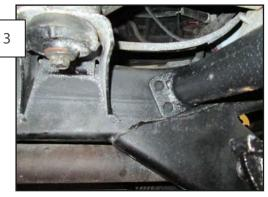
Position the rear, angled, plate against the rear of the frame; just above the rear control arm frame mount. Hold the guard and measure the guard from the body pinch weld, to ensure it is parallel with the vehicle. Measure the vertical position from the body/frame mounts and match the measurements on the opposite side of the vehicle.
