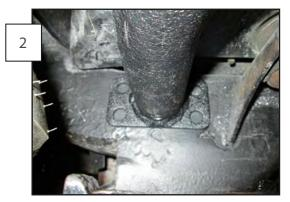
hold one of the guards level with the jeep body and position the front, horizontal, plate against the frame.
