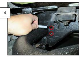
While the guard is still parallel with the vehicle body, mark each of the 8 holes with a marker. Remove the guard and drill 1 5/16" hole at each mark. Insert the included screws and thread them into the predrilled holes. Be sure not to drill the hole too large for the threads.
