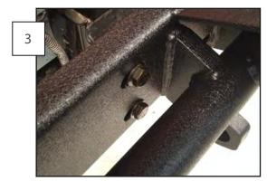
Place the new bumper over the front of the vehicle frame and insert the 4 inner bolts into the holes from the front. Attach a lock nut to the back and tighten them.
