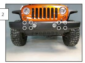
Remove the 4 nuts on the backside of the bumper that attach the front bumper to the frame.
