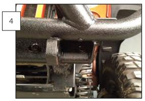
Insert the 4 outer bolts into the holes from the front. Attach a lock nut to the back and tighten them. Secure any fog light wiring out of sight and away from moving parts.
