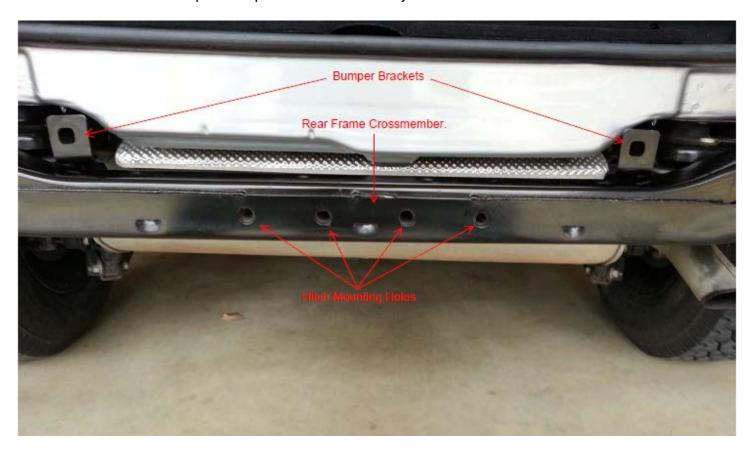
4. Locate the hitch mounting hardware. The hardware should consist of 4- bolts, 4- lock nuts, and 8- flat washers.
