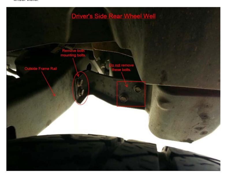
3. Remove the rear bumper and place it out of the way.
