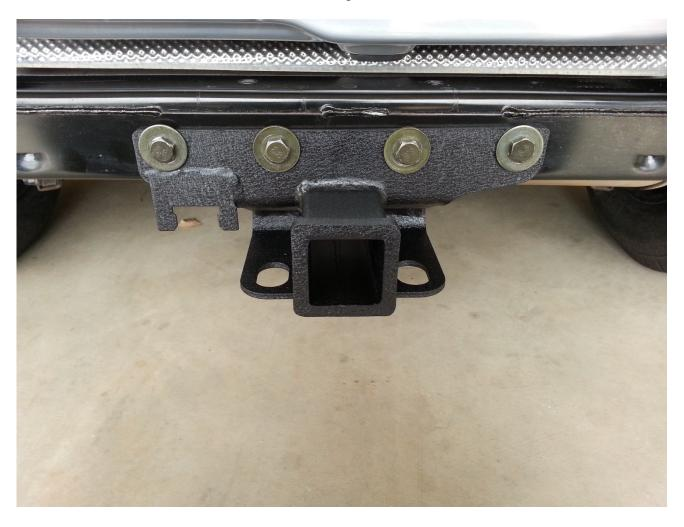
8. Reinstall the rear bumper in the reverse order it was removed. Do not tighten the hardware until the bumper is properly positioned.
