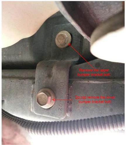
2. Remove the mounting bolts connecting the bumper to the outside frame rail on both the driver and passenger sides. There are 2- 15mm bolts on each side. The bolts are accessible from the rear wheel wells.
