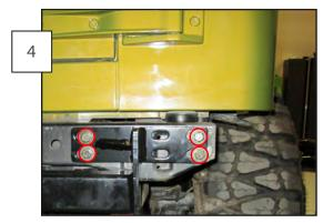
Install the hitch to the frame with 4 of the bolts included with the hitch. use a washer on both the bolt head side and the nut side. Install a lock washer on the nut side, then tighten each connection. The large hardware and two hole plates are for installation of a tube bumper to the
