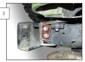
Remove the (2) rear bumper to frame nuts. Repeat on the opposite side.
