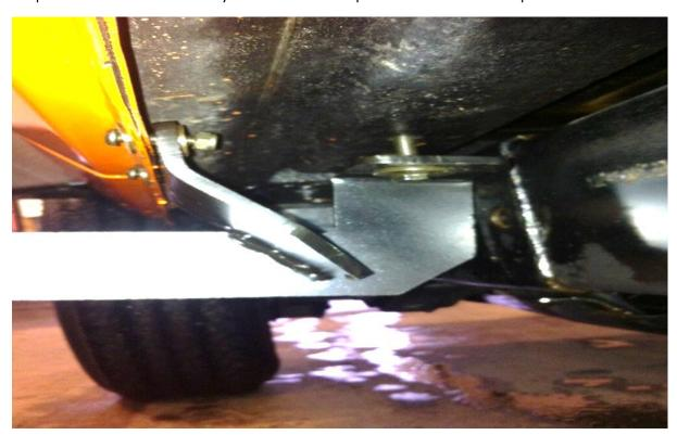
3. After you have installed both brackets find the left and right side steps; install 2 bolts with LOCK washers and washer through the brackets into the threaded bottoms of the side steps. Now adjust steps to desired position. Make sure to twist side steps so they are level.
