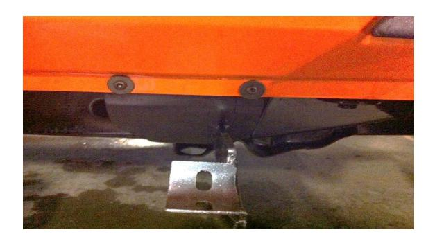
2. Insert a large bolt with a washer. If you have a 2011 or older you will need to insert a nut plate. 2012 and newer have pre-treaded holes in the body. Remember to keep bolts loose until last step.
