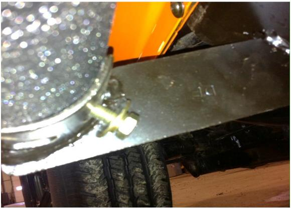
4. Now that side steps are in position tighten down all hardware on body then tighten down the steps in place. You might need to readjust by twisting side steps to be level before tighten.
