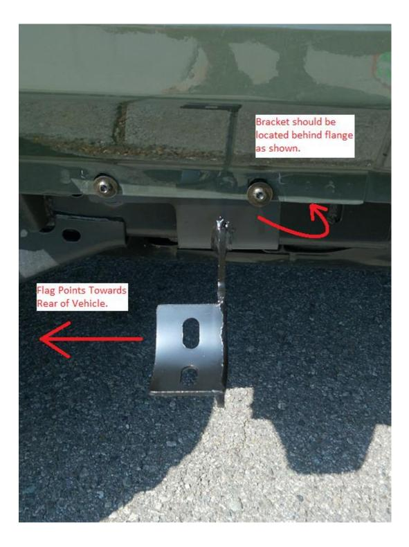
5. Use the 8-1.25 mm x 35mm nuts and washers to secure the brackets. Loosely secure the nuts using the 10mm socket with a wrench.
