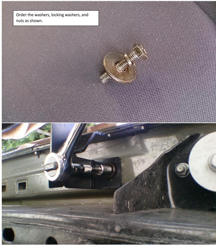
6. In case there are no threaded inserts on the bottom of your vehicle, there should be an opening that will allow for the use of nut plates. Use these to secure the brackets with the 10-1.5mm nuts and 13mm socket wrench.
