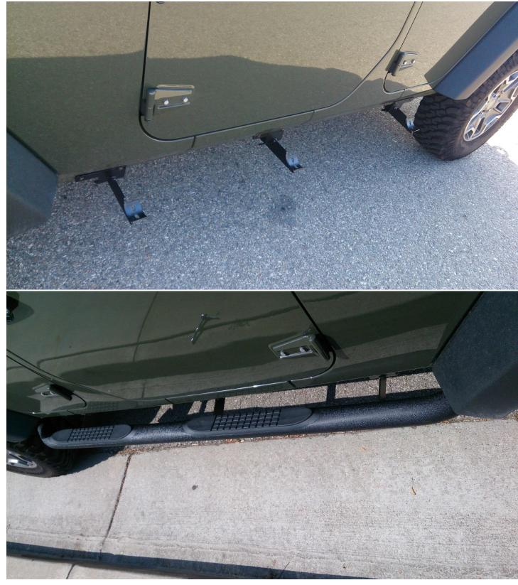
9. Use the remaining 8-1.25mm x 25mm bolts and washers to secure the side steps to the brackets. Use a 10mm Socket wrench to secure.
