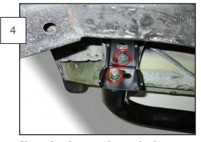
Place a bracket over the rear body mount. Reinstall the stock body bolt through the outer oval hole in the bracket. Tighten the bolt until it loosely holds the bracket in place.
