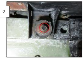
Remove the (2) 16mm factory body bolts, located between the wheels, on one side of the Jeep. (Only remove one side at a time.)
