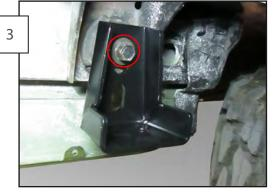
Place a bracket over the front body mount. Reinstall the factory body bolt through the inner oval hole in the bracket. Tighten the bolt until it loosely holds the bracket in place.
