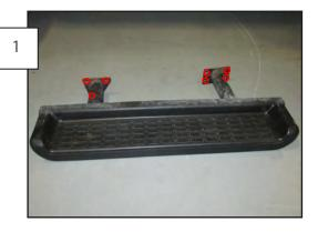
If your Jeep came with a factory step, start by removing the (7) 10mm bolts where the steps attach to the frame. Remove the factory step and repeat on the other side.
