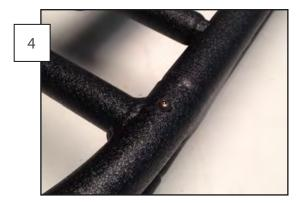
Carefully turn the basket over and install an allen head screw, with a washer, at each pre-drilled hole; where the end pieces meet the side rails. Turn the basket back over and prepare to place it on the Jeep roof rack.
