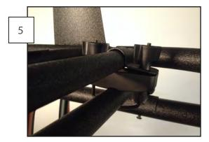
Lay the basket on top of the roof rack and install the plastic spacer between the rack and the basket's end piece cross brace. Install the clamp over the rack, through the plastic spacer and the metal hoop. Tighten down all 4 corners of the rack until they are tight.
