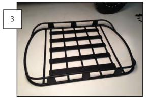
Install the second end piece onto the 2 side rails. Then, lay the horizontal pads across the horizontal rails. Line up the rail screw holes with the pad screw holes, then tighten down 1 whole pad; this will line up the rest of the pad holes, vertically, to install the rest of the pads and screws.
