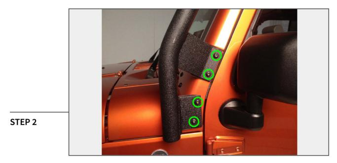
Remove the (4) drivers side T40 torx bolts on both sides of the windshield and install the vertical support.
