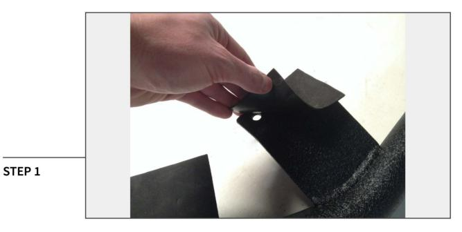
Remove the backing and apply the adhesive side of the included rubber padding to the inside of the vertical windshield support plates that attach to the windshield frame.
