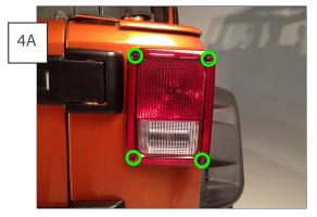
REAR BODY MOUNT ONLY: Remove the 4 tail light screws and remove the tail light from the vehicle.
