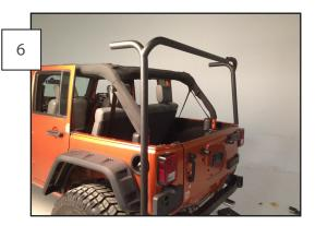
Insert the rear light bar into the vertical support, secure it with an allen head screw. Install the other vertical support the same way and insert the rear light bar into the slip fitting.
