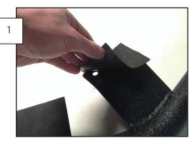
Remove the backing and apply the adhesive side of the included rubber padding to the inside of the vertical windshield support plates that attach to the windshield frame.
