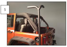
Install the rear vertical support into the rear vertical frame support or body bracket. Secure it with an allen head screw.
