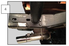
IF ATTACHING TO THE REAR FRAME: Remove the aftermarket rear bumper. Attach the rear vertical support to the frame utilizing (2) of the included hex head bolts inserted into the two existing bumper support holes left from the stock bumper. (2) shims, with 3 holes, are provided if the aftermarket bumper is externally mounted. IF BODY MOUNTING SEE STEP 4A.
