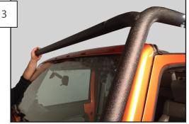
Insert the horizontal windshield light bar into the vertical winshield support that was installed in step 2. Have someone hold the free end or rest it on a rag, while inserting an allen head screw into the pre drilled hole on the slip joint. Install the passenger side vertical windshiled support the same way the drivers side was installed in step 2. While installing it, slide the horizontal winshield light bar into the vertival windshield support.
