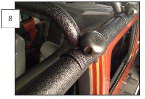
Lay a luggage support bar across the top of the vehicle and secure both sides with a long allen head and a knob nut. Repeat this for the other luggage support bars.
