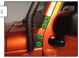
Remove the (4) drivers side T40 torx bolts on both sides of the windshield. Install the vertical support.
