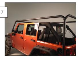
Insert the side rails into the front and rear vertical supports, secure them with an allen head screw. Secure the rear slip fit with an allen head bolt, then repeat the process on the other side. Make sure the holes point from the upper outside to the lower inside.
