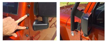
Slide front Cross Bar into partially installed first side Front Leg and secure it with the (1) 8mm x 65mm Allen Bolt,
