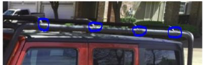
12. Go back over and tighten all connections and snugging all bolts and screws to ensure minimal vibrations. The end result is upon you!
