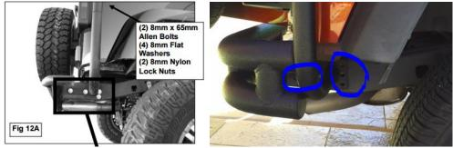
11. Locate the shortest Cross Rail and position it over the mounting bolt holes toward the front of the Side Rails. Secure the Basket Holder Cross Rails to Side Rails by inserting (1) 8mm x 70mm Allen Bolt with (1) 8mm Flat Washer up through the bottom hole in the Side Rail and through Cross Rail and placing (1) 8mm Flat Washer over each bolt and secure it with included 8mm Nylon lock nuts.
