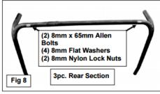
8. With assistance, attach the assembled rear top section of the Roof Rack to the already inserted Side Rails. Use the included (2) 8mm x 65mm Allen Bolts, (4) 8mm Flat Washers and (2) 8mm Nylon Lock Nuts to attach the Rear Top Legs to the Side Rails.
