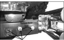
Slide both side rails, (with top holes angled towards the outside of the vehicle), into the previously installed front legs. Secure the side rails to the front legs using the included (1) 8mm x 65mm Allen Bolt, (2) 8mm flat washers and (1) 8mm nylon lock nut. Do not tighten hardware!!
