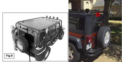
9. With assistance, hold the rear section of the Roof Rack up and attach the Rear Bottom Leg section to the Rear Top Leg sections using the included (2) 8mm x 65mm Allen Bolts, (4) 8mm Flat Washers and (2) 8mm Nylon Lock Nuts.
