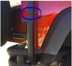
10. Position the passenger Rear Bottom Leg up to the frame and align the holes in the Bracket with holes in the frame for the bumper. Secure the rear holes in the Mounting Bracket to the bumper using the same bolts that came with your aftermarket bumper. Attach the front of the Bracket to the frame using the factory bolts or the included hardware. Repeat this step for the driver side installation.
