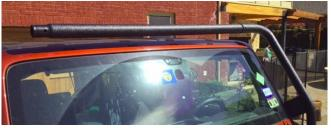
3. As in Step 1, Use your TX40 Torx bit and socket to remove the passenger side windshield hinge bolts and attach the passenger side front leg using (4) 8-1.25mm x 35mm hex bolts, (4) 8mm Lock Washers and (4) 8mm x 24mm OD x 2mm Thick Flat Washers. Proceed to secure upper section of the front leg to front Cross Bar using the included (1) 8mm x 65mm Allen Bolt, (2) 8mm Flat Washers and (1) 8mm Nylon Lock Nut.
