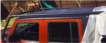
6. To better support the Roof Rack when loaded, (2) Rubber Bumpers are included in the installation kit. The Rubber Bumpers can be installed at a point 29" up from the end of the Rear Leg for vehicles with hard tops or at 6-3/8" for vehicles with hard or soft tops. You will need to measure, then drill a 1/8" hole into the Rear Leg at the desired height. Secure the Rubber Bumper to the Rear Leg with (1) #5 x 30mm Screw and (1) 5mm Flat Washer.
