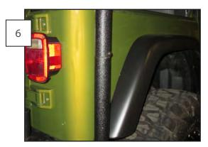
Install the upper rear vertical support into the lower rear vertical mount. Install a medium 5mm Allen bolt, washer / washer, lock nut combination to hold it in place. These are side specific and will curver in toward the body from bottom to top.
