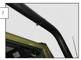
Install a side horizontal support into the front vertical support and loosely install a medium 5mm Allen bolt, washer / washer, lock nut combination to hold it in place. Be sure to support the rear of the support to keep it from damaging the vehicle.
