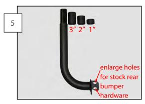
IF THE VEHICLE IS EQUIPPED WITH BODY SPACERS: Use the supplied roof rack vertical spacers on the rear vertical mount. They are measure for 1"-3" body lifts and will lift the rear of the rack to compensate for the difference.
