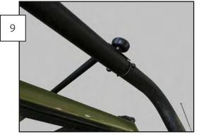
Install the (1) short cargo support bar into the front holes of the rack, then the (2) longer bars into the rear holes. Place included adhesive foam to the lower side of the cargo support bars. Install the cargo support bars on the horizontal supports and connect them with 5mm Allen bolts, washers / hand knobs (as shown). Make sure the roof rack is sitting straight and tighten down all hardware.
