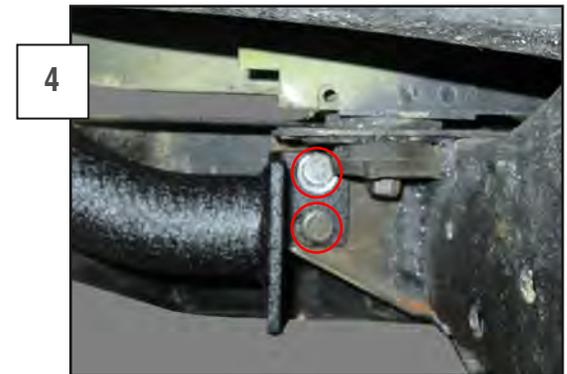
Reinstall the rear bumper hardware through the lower rear vertical mount and snug the hardware, leaving approximately a 1/4" of play for install. Use the (4) included hex bolts and nuts if needed.
