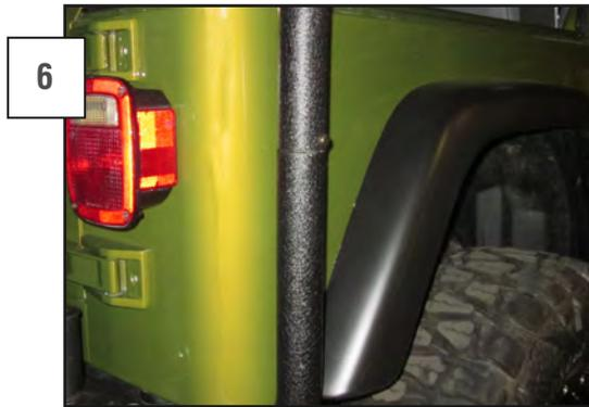
Install the upper rear vertical support into the lower rear vertical mount. Install a medium 5mm Allen bolt, washer / washer, lock nut combination to hold it in place. These are side speci c and will curver in toward the body from bottom to top.
