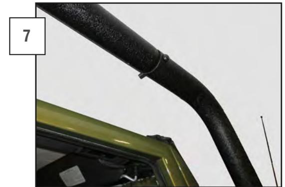
Install a side horizontal support into the front vertical support and loosely install a medium 5mm Allen bolt, washer / washer, lock nut combination to hold it in place. Be sure to support the rear of the support to keep it from damaging the vehicle.
