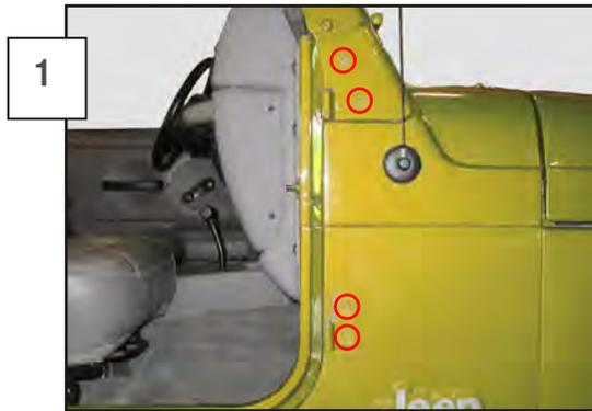
Remove the door from the vehicle. Remove the (4) stock T40 screws from the upper and lower hinge. The lower hinge will separate from the body and a threaded plate on the inside of the vehicle will also separate.
