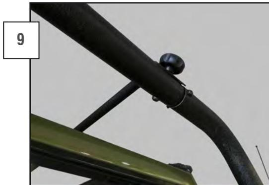
Install the (1) short cargo support bar into the front holes of the rack, then the (2) longer bars into the rear holes. Place included adhesive foam to the lower side of the cargo support bars. Install the cargo support bars on the horizontal supports and connect them with 5mm Allen bolts, washers / hand knobs (as shown). Make sure the roof rack is sitting straight and tighten down all hardware.
