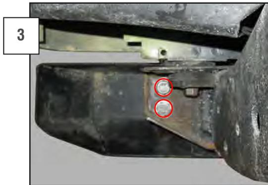
Support the rear bumper. Remove the (2) rear bumper mounting nuts or bolts. If you are reusing the stock bumper the holes shown in figure 5 will need to be enlarged.
