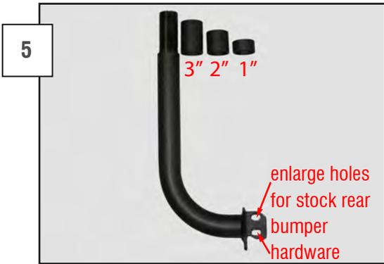
IF THE VEHICLE IS EQUIPPED WITH BODY SPACERS: Use the supplied roof rack vertical spacers on the rear vertical mount. They are measure for 1"-3" body lifts and will lift the rear of the rack to compensate for the di erence.
