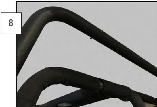
Maneuver the rear vertical support onto the horizontal support and install a medium 5mm Allen bolt, washer / washer, lock nut combination to hold it in place. Repeat these steps on the opposite side of the vehicle.
