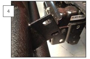
Place the bumper onto the brackets by sliding the lower corner of the bumper plate onto the top corner of the bumper bracket. It is a tight fit, but it will slide into place.
