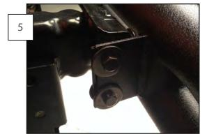
Make sure the bumper is level and tighten down the two outer bumper and bumper bracket bolts. Use washers on both the bolt and nut side of each hardware connection.
