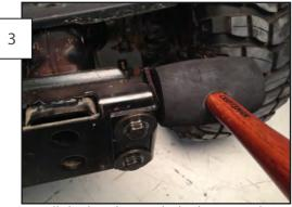
Install the bracket, with the horizontal holes againsts the front of the vehicles frame holes. The bracket should bend toward the rear of the vehicle. Tighten down the two bracket to frame bolts and hit the top of the bracket with a mallet to angle it in slightly at the top.
