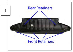
Remove the 4 front and 2 rear, plastic push pin, splash shield retainers. Remove splash shield from the vehicle.
