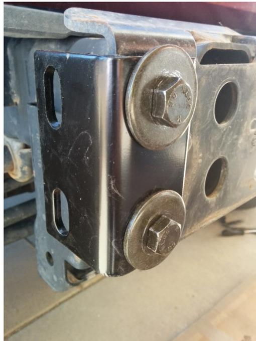
4. Place the bumper onto the brackets by sliding the bottom of the bumper mount onto the top corner of the frame mount. It will be tight but continue to apply pressure downward and slide it into place.
