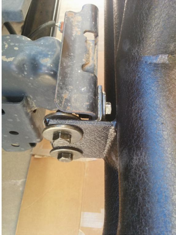
5. Once you have the bumper level, go ahead and tighten the bolts using the 18 mm socket on the head side and the 19 mm wrench on the nut side. Make sure that you use a flat washer on both the head side and the nut side
