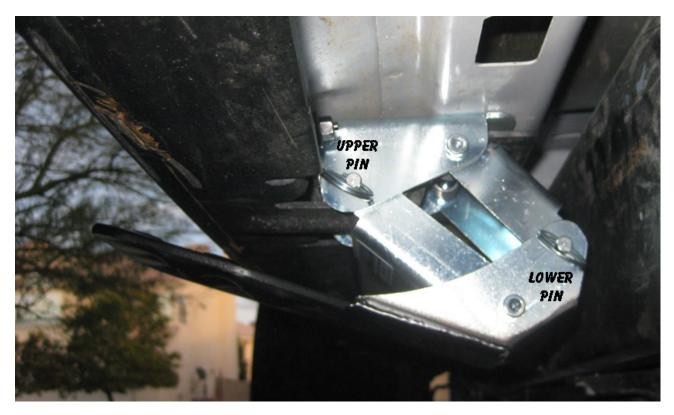
7. The finished product works beautifully. When folded up it only sticks out about an inch from the body but still provides adequate sufficient area to grab onto. When extended there is plenty of room for my size 11 shoe.
