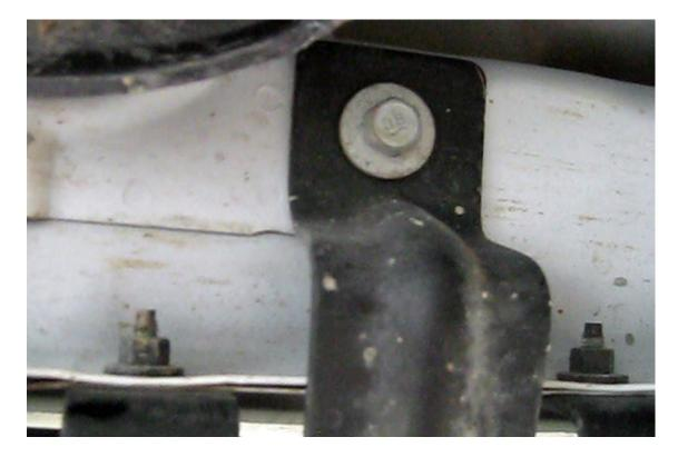
9. Connect the step to the step base using the removable pins supplied with the kit. NOTE: An installation video from M.O.R.E. suggests wedging a hammer handle or something behind the spring loaded side of the step base to facilitate lining up the holes to insert the upper pin.
