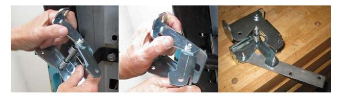
6. Temporarily slide the step base into position. The step base plate goes between the body of the jeep and the rocker guard mounting arm.
