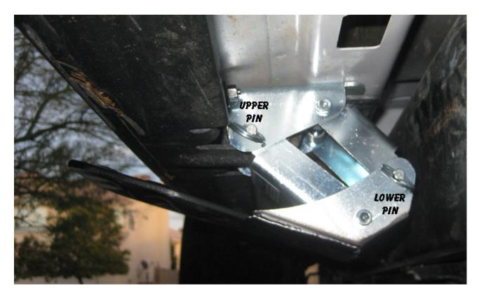
10. The finished product works beautifully. When folded up it only sticks out about an inch from the body but still provides adequate sufficient area to grab onto. When extended there is plenty of room for my size 11 shoe.
