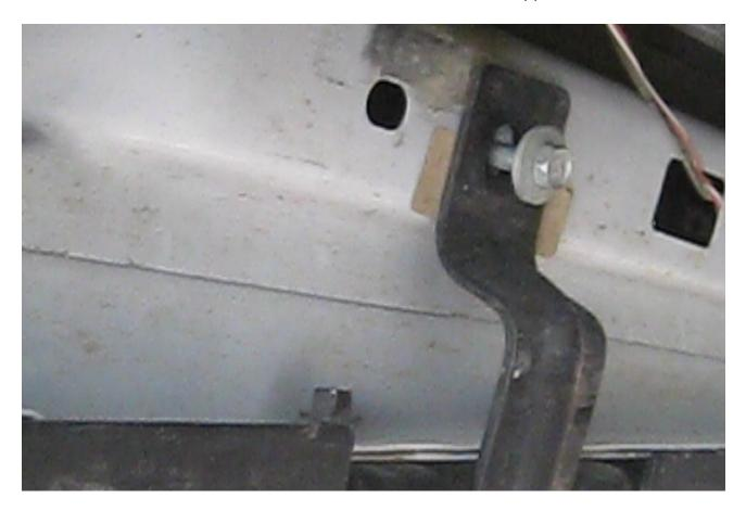
3. Take a pry bar and bend the connecting arm down about ¼ inch so that the step base can easily slide under it.
