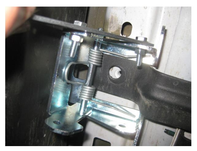
7. If the slots in step base do not line up with the 2 studs in the pinch seam you'll have to enlarge the holes and/or bend the base plate to make it fit. WARNING: Make sure there is sufficient clearance for the upper pin to clear the rocker guard mounting arm. I had to insert an additional washer as a shim between the step base plate and the rocker guard mounting arm to provide enough clearance.
