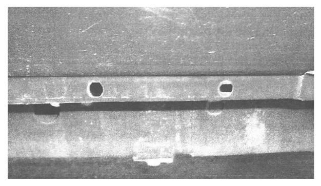
4. Install the u-nut into the hole in the body directly behind the 2 holes in the pinch seam.
