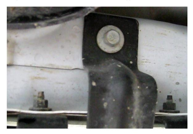
5. Compress the spring to bend the step base approximately 90 degrees. Use the metal strap and small bolts to hold it in that position while you go through the installation process.
