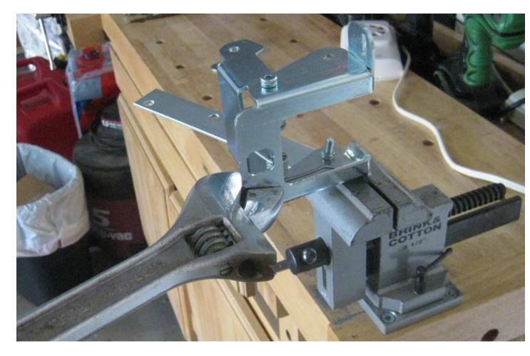
8. Once you are satisfied with the fit, reinstall the 2 nuts onto the studs, then install the 13mm bolt using the large washer supplied with the kit.
