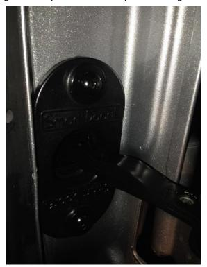
21. Secure the pivot arm of the hinge assembly to the hinge plate by replacing the Torx nut and using your Torx Socket T50 to tighten it. Do not over tighten the nut until you have tested the door to make sure that it opens and closes properly without binding. Do not force the door – make adjustments to ensure smooth operation.
