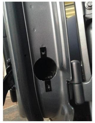
17. Test to make sure the nuts, door holes, and hinge assembly all line up properly before final tightening. Insert the hinge assembly into the hole, ensuring the when doing the left door that the "L" is facing up. Likewise, when doing the right door, make sure that the "R" is facing up.
