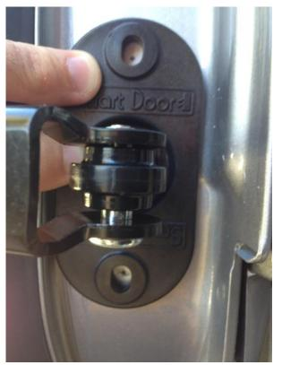
13. Remove the hinge assembly and drill the two additional holes using a 5/16" bi-metal drill bit.
