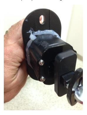
20. Insert the hinge assembly into the hole, ensuring the when doing the left door that the "L" is facing up. Likewise, when doing the right door, make sure that the "R" is facing up. Use the 5/32" Allen Wrench to tighten the 1" screws into the hinge assembly holes and the clip on nuts. Tighten firmly, but not to full strength yet.
