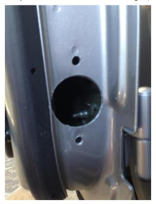
14. (Optional Step) File the rough edges of the openings and vacuum up the metal shavings.
