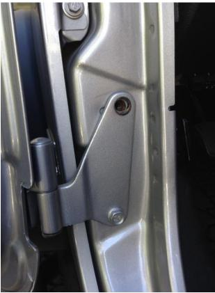
6. Place the Star Fabricating hinge plate over the Jeep's hinge plate, and secure it in place with the Star Fabricating 13mm replacement bolt. Do not over tighten the bolt – just make sure it is firmly in place. (Optional: If you have a second 13mm socket, you can place it through the bottom hole of the Star Fabricating hinge plate and onto the Jeep's 13mm lower bolt to keep the Star Fabricating hinge plate in place.)
