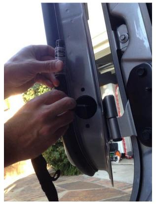
16. Attach the clip on nuts to the upper and lower holes. I accidentally dropped one of the nuts into the door, but retrieved it using a telescoping magnet. If the clips are too tight, pry them open a bit with pliers and a regular screwdriver.
