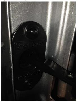
19. Once you are sure that the screws and nuts will properly align, remove the screws and the hinge assembly. Place a bead of Silicone sealant completely around the hinge's backside to create a water tight seal.
