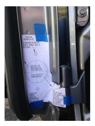
10. Mark the three drilling locations by placing the center punch (or Phillips head screw driver) on the spot and hitting it with your hammer.
