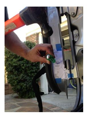
11. Remove the template and drill the two-inch hole in the center marking using the 2" Bi-Metal hole saw. Now Stop! Do not drill the other two holes until you have ensured everything lines up.
