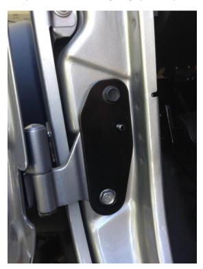
7. Remove the bottom bolt on the Jeep's lower door hinge. Replace it with the Star Fabricating washer plug and 13mm replacement bolt. Do not over tighten the bolt – just make sure it is firmly in place.
