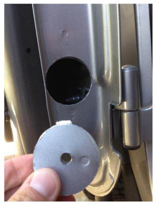
12. Insert the Star Fabricating Smart Door Hinge into the new two-inch hole. Make sure that your marks for the two additional holes are centered up in the openings of the hinge assembly. Assuming that you were meticulous in cutting out the templates, taping them to the door, and marking the drill points with a center punch, your drill markings should be perfectly placed.
