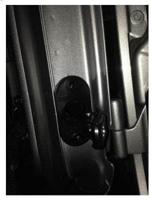
18. Use the 5/32" Allen Wrench to tighten the 1" screws into the hinge assembly holes and the clip on nuts. This was the trickiest and most challenging part of the installation. If the screws do not align properly with the opening on the clip on nut, you will not be able to secure the hinge assembly. I tried using different angles (top to bottom or bottom to top), and I was able to get the screws in on the first door.
