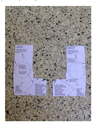
9. Fold the template where it says, "Fold up at this edge." Carefully tape the template in place on the door. Double check that the template is properly positioned at all indicated marks. Ensure that the two-inch circle in the center of the template is centered up on the door wall as this will be where the two-inch hole will be drilled.
